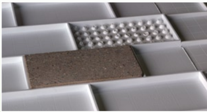
8" x 16" blocks placed in VersaLiner.
